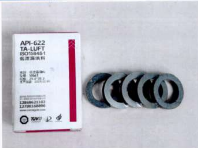
试验前的填料环 Packing rings before test
