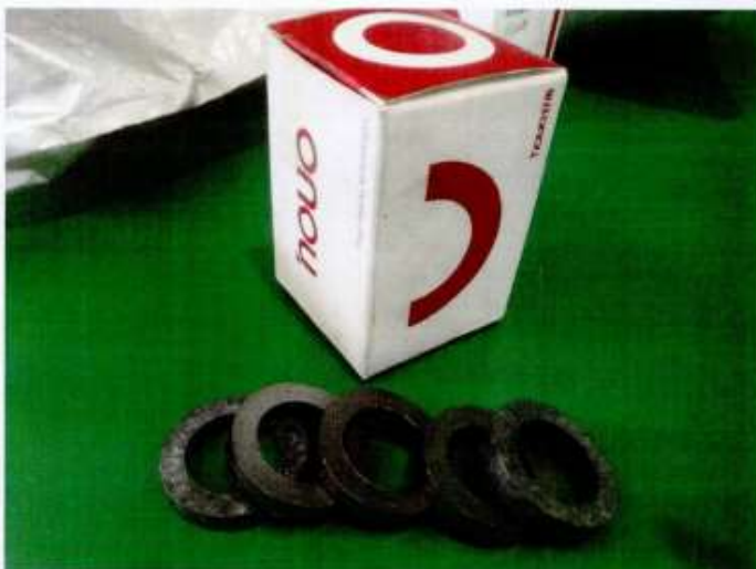
试验前的填料环 Packing rings before test
