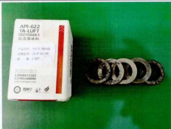
试验后的填料环 Packing rings after test
